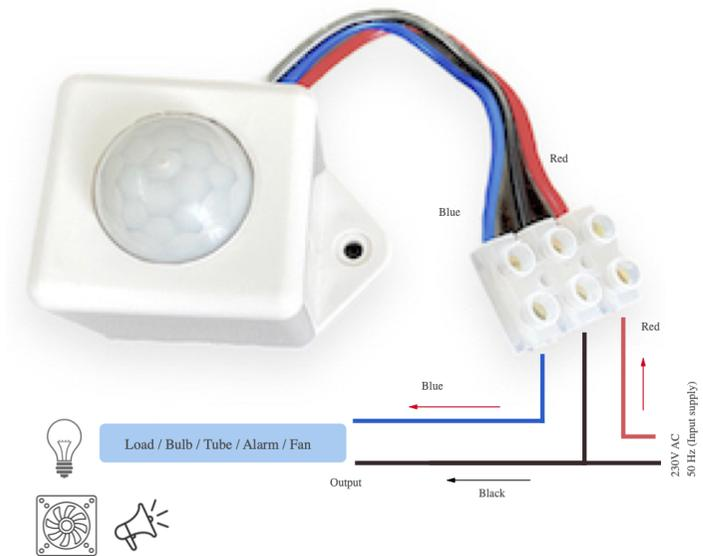
Black wire is common, the Red wire is line input voltage and Blue must be connected to load.
