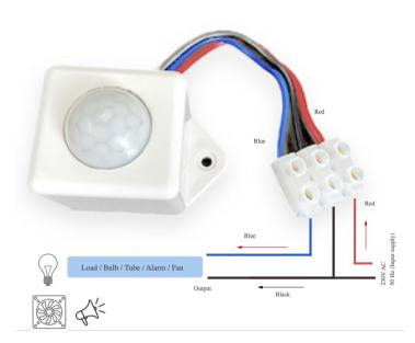
Black wire is common, the Red wire is line input voltage and Blue must be connected to load.
